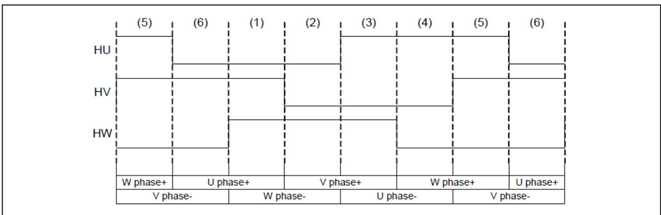
If the conduction patterns of each phase are changed in the switching timing of these hall sensor signals, as shown in Figure 3-2, rotating flux generated as shown in Figure 3-3. Then the rotor has the torque and rotates.
