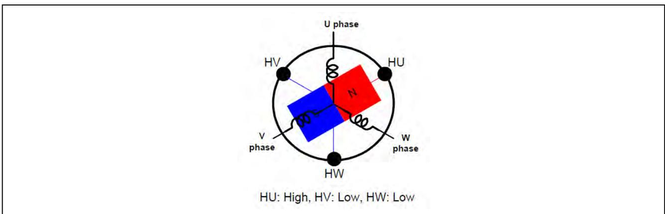
As shown if Figure 3-1, a hall sensor is allocated every 120 degrees and the respective hall sensor signals are switched depending on direction of rotating magnetic poles. Position information can be obtained every 60 degrees (six patterns for one cycle) by combining these three hall sensor signals.
