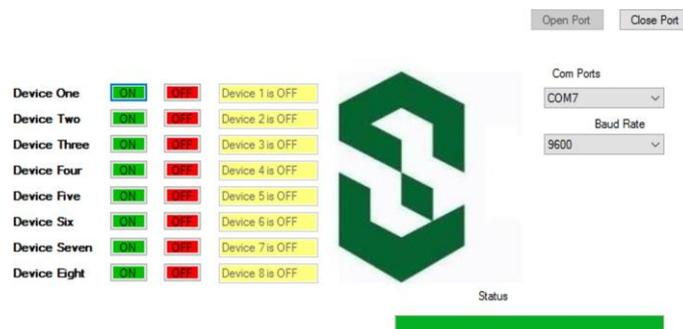
Figure 8. Visual C# Application for Receiving/Sending Data to/from consumer
