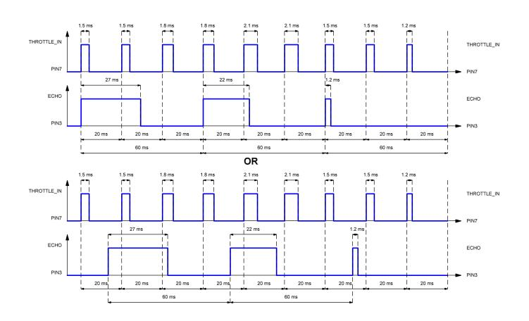
Figure 7. Collision Avoidance Controller ECHO and THROTTLE\_IN signals
