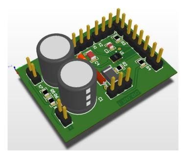
Figure 3. Collision Avoidance Controller PCB illustration
