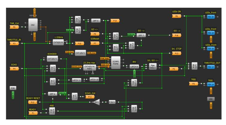
Figure 5. Collision Evasion Controller circuit design (Matrix 1)
