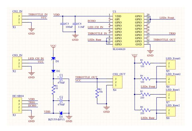
Figure 2. Collision Avoidance Controller schematic example
