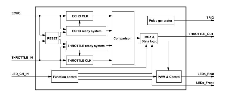
Figure 6. Block Diagram
