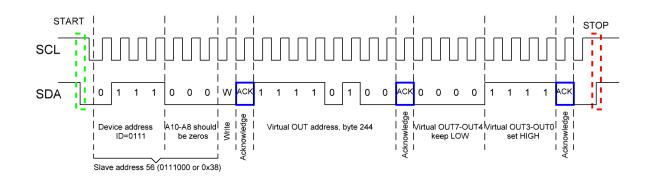
Fig. 2. ACMPs powering up via I2C programming of Virtual OUTs. Timing Diagram
