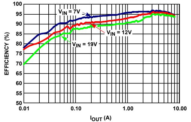
**FIGURE 6. CHANNEL 2 EFFICIENCY AT  $V_O = 5V$ , DEM OPERATION. HIGH-SIDE 1xIRF7821,  $r_{DS(ON)} = 9.1m\Omega$ ; LOW-SIDE 1xIRF7832,  $r_{DS(ON)} = 4m\Omega$ ;  $L = 4.7\mu H$ ,  $DCR = 14.3m\Omega$ ; CCM  $F_{SW} = 330kHz$**
