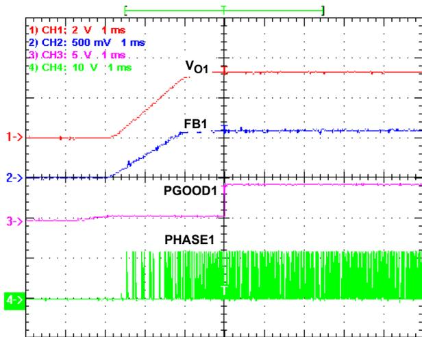
**FIGURE 7. POWER-ON,  $V_{IN} = 12V$ , LOAD = 5A,  $V_O = 3.3V$**
