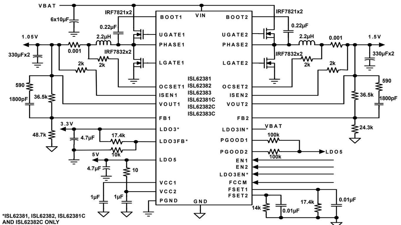
FIGURE 4. TYPICAL APPLICATION CIRCUIT WITH RESISTOR CURRENT SENSE
