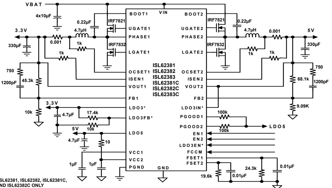
FIGURE 2. TYPICAL APPLICATION CIRCUIT WITH RESISTOR CURRENT SENSE
