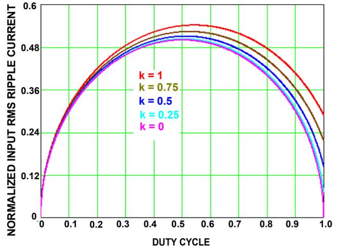
FIGURE 28. NORMALIZED RMS INPUT CURRENT @ EFF = 1
