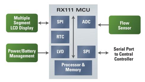
Figure 2: Flow meter example application
