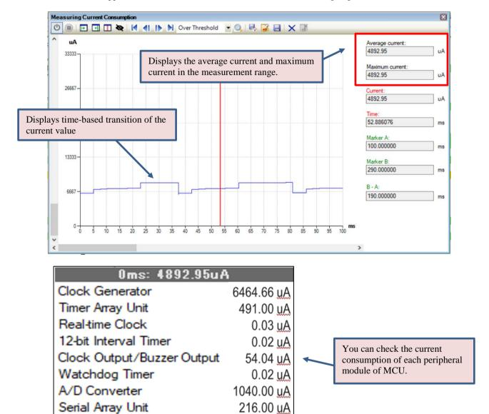
Figure 2-3 Measurement results of current consumption simulation
