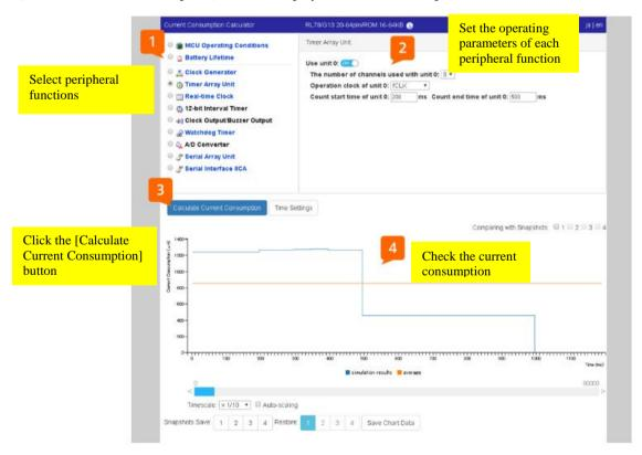
Figure 3-1 Example of Current Consumption Calculator Window
