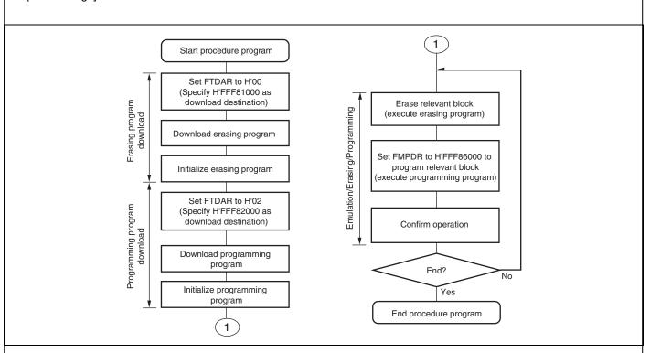
Page 933, (4) Erasing and Programming Procedure in User Program Mode, 2. Be sure to initialize both the erasing program and programming program.
