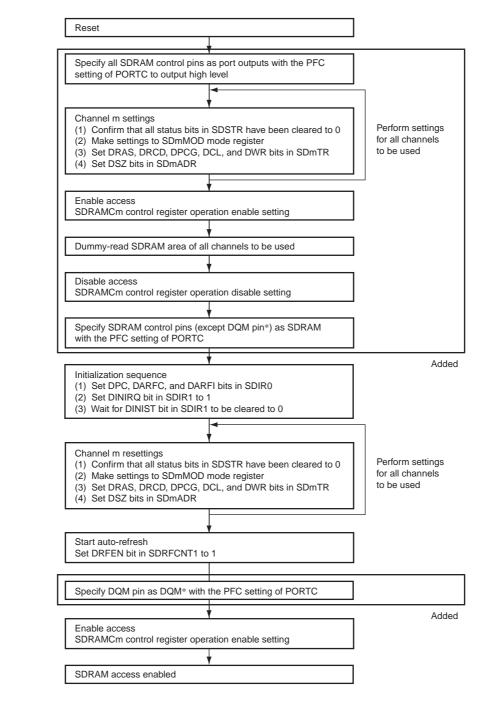
Note: \* It is recommended that the DQM pin be driven high before the initialization sequence for some SDRAM. In this case, the setting may be necessary.
