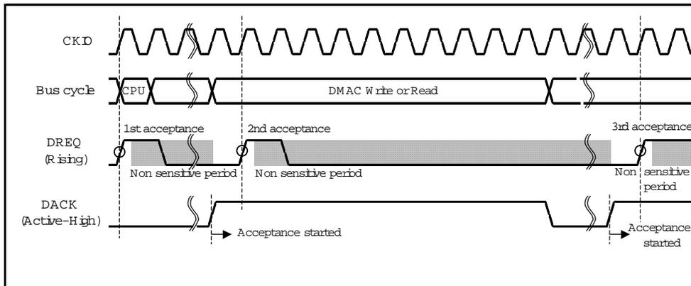
Fig2. Example of DREQ Input Detection in Cycle Steal Mode Edge Detection
