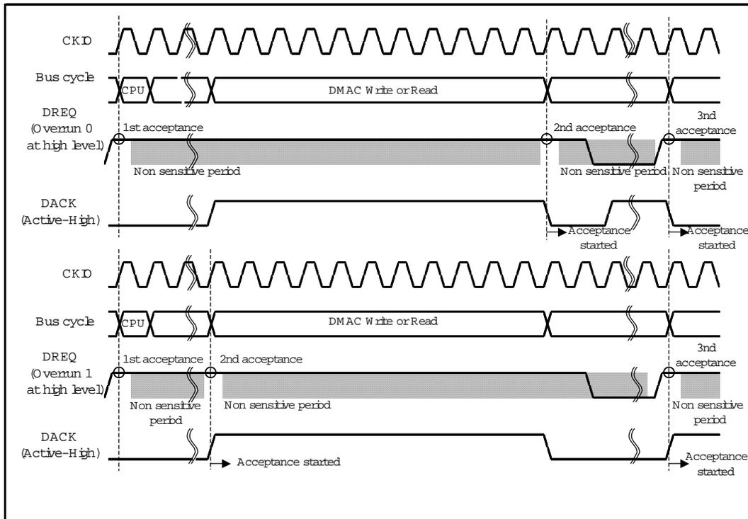
Fig4. Example of DREQ Input Detection in Cycle Steal Mode Level Detection
