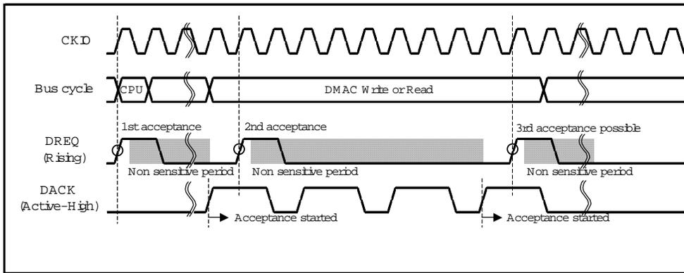
Fig1. Example of DREQ Input Detection in Cycle Steal Mode Edge Detection
