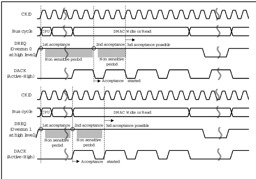
Fig3. Example of DREQ Input Detection in Cycle Steal Mode Level Detection
