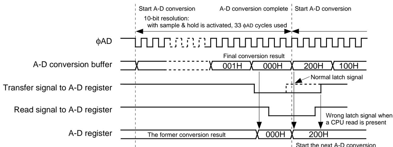
Normally, A-D conversion value is saved at the rising edge (dashed rising edge) of the latch signal. However, when the CPU is doing a read to A-D register at this time, the A-D register latch signal is delayed, and wrong value is stored at A-D conversion register.
