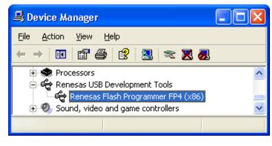
If the programming GUI for the PG-FP4 is started-up in state 2, "E307 Trying to open USB failed" appears, and it will not be detected.
