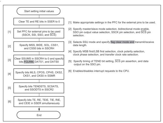
Figure 15.4 Example of Initial Settings in SSU Mode
