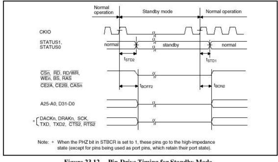
Figure 23.12 Pin Drive Timing for Standby Mode
