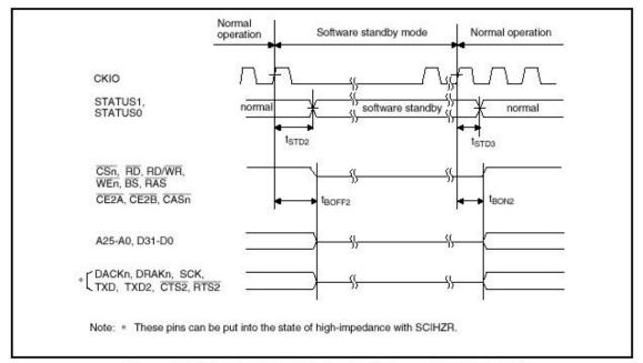
Figure 23.12(2) Pin Drive Timing for Software Standby Mode
