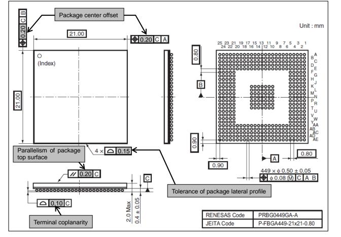
Figure E.1 Package Dimensions (449-Pin BGA)
