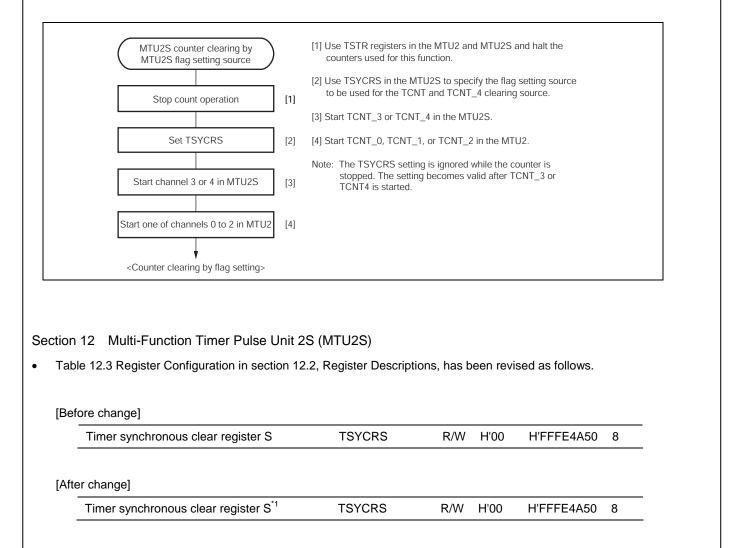
\*1 For details on registers, refer to section 11.3.9, Timer Synchronous Clear Register (TSYCR) and figure 11.85 in section 11, Multi-Function Timer Pulse Unit 2 (MTU2).
