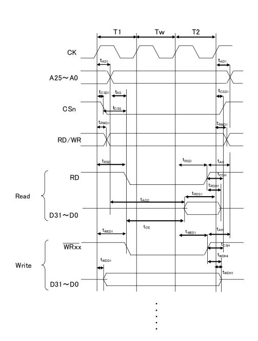
Figure 31.12 Normal Space Basic Bus Cycle (Software Wait 1)
