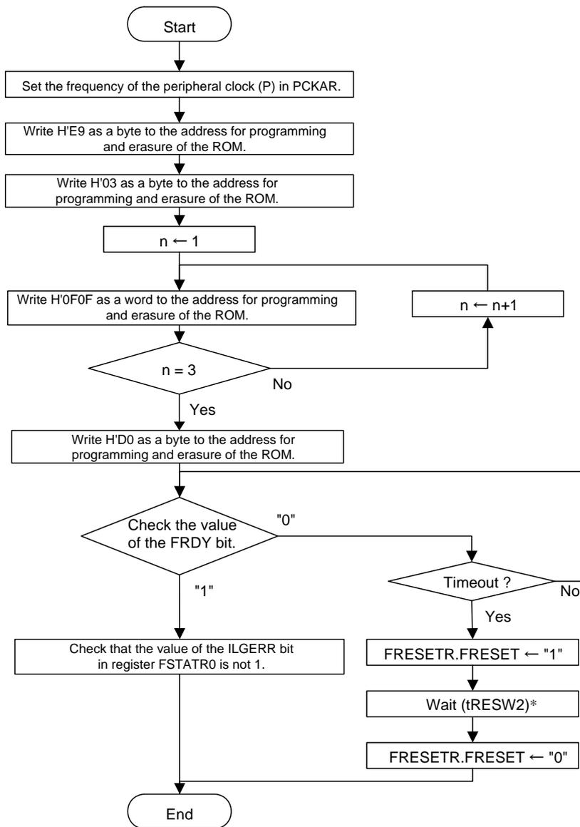
Note: tRESW2 denotes the width of a reset pulse during programming or erasure (see section 33.3.2, Control Signal Timing, in section 33, Electrical Characteristics).
