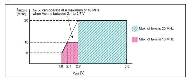
Figure 1. Relation between  $f_{(BCLK)}$  and  $V_{CC1}$
