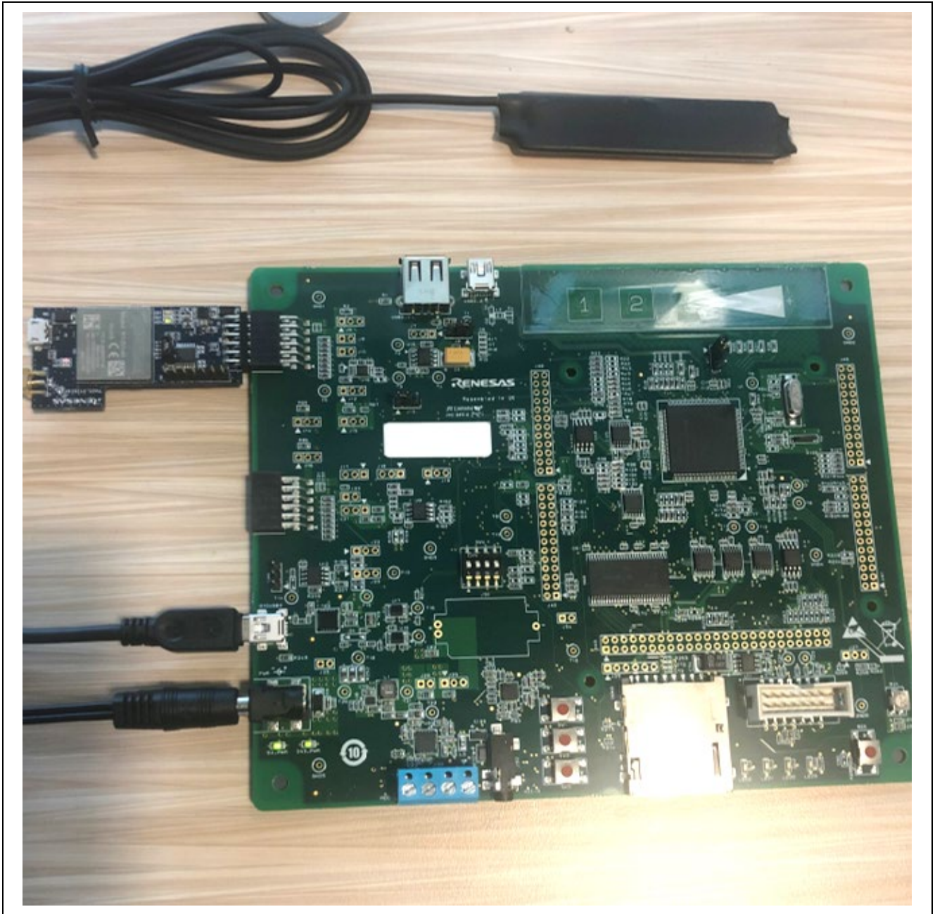
Figure 4. Connections for the RX671 Board After Flashing
