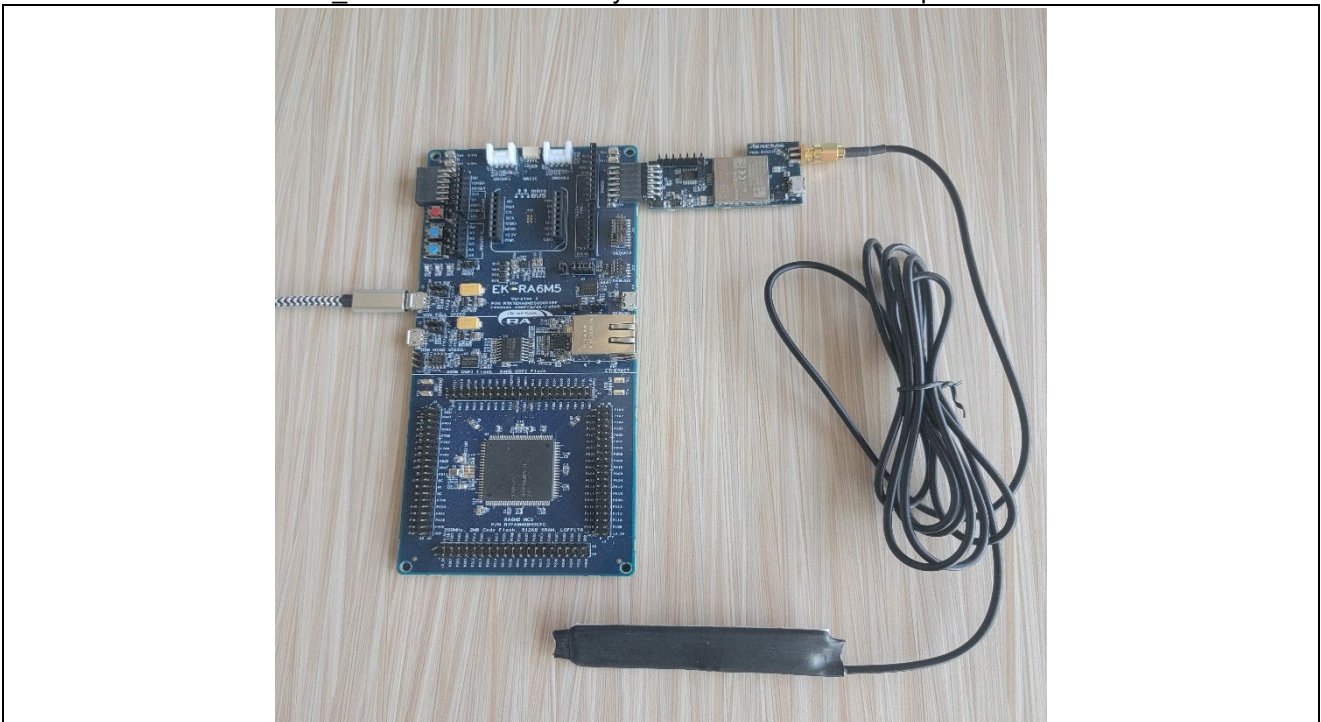
Figure 1. EK-RA6M5 Setup with RYZ014A_PMOD Module Connected
