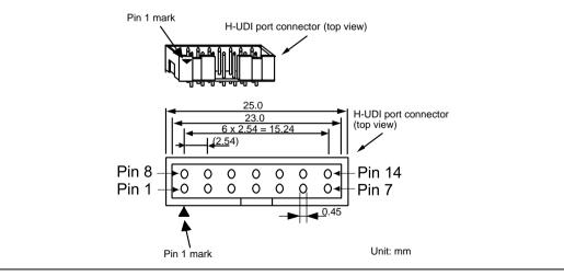
Figure 1.2 Pin Assignments of the H-UDI Port Connector (14 Pins)
