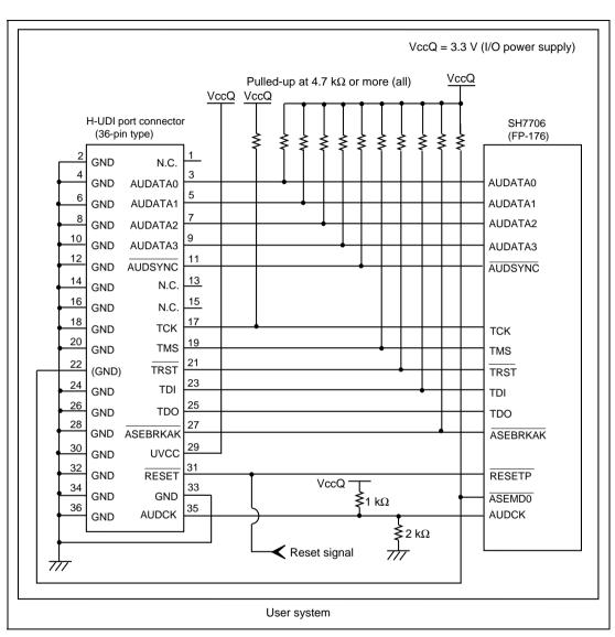
When the circuit is connected as shown in figure 1.3, the switches of the emulator are set as SW2 = 1 and SW3 = 1. For details, refer to section 3.8, Setting the DIP Switches, in the Debugger Part of the SuperH<sup>TM</sup> Family E10A-USB Emulator User's Manual.
