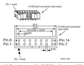
Figure 1.2 Pin Assignments of the H-UDI Port Connector (14 Pins)
