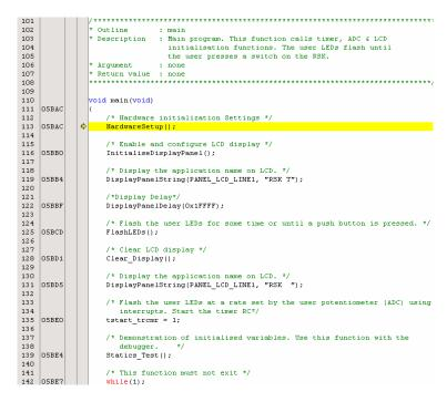
• Place an event at the call to InitialiseDisplayPanel(); by double clicking in the On-Chip Breakpoint column next to the line to stop at.
