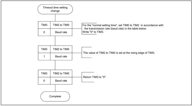
Figure 9.8 Normal Setting Time  $\rightarrow$  Initial Setting Time
