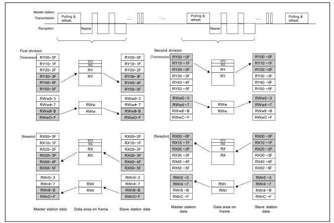
Figure 11.1 With 2 Occupied Stations and Extended Cyclic 2 × Setting
