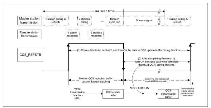
Figure 13.1 Link Scan Time and CCS\_REFSTB Signal Change
