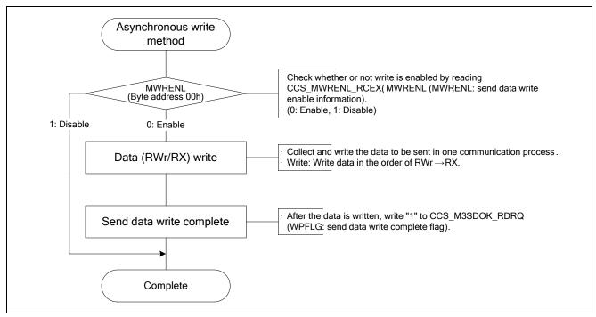
Figure 9.6 Asynchronous Write Method
