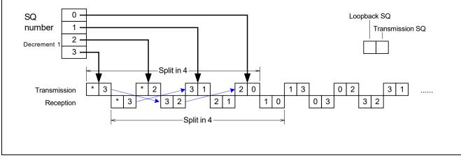
Figure 11.5 Details of SQ Value (Loopback)
