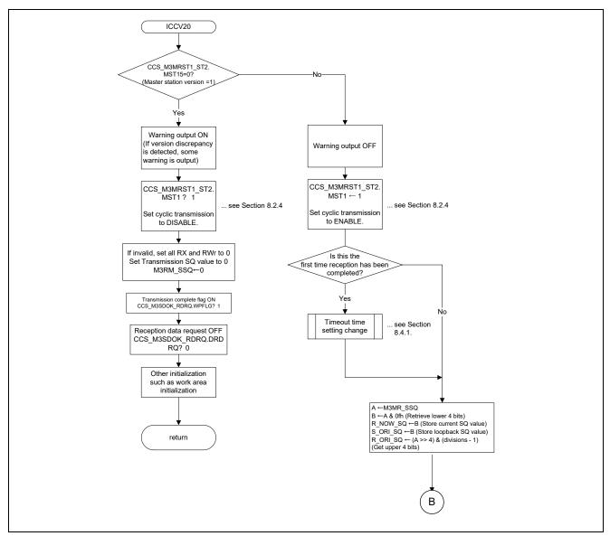
Figure 12.4 Transmission/Reception Processing Module (ICCV20)
