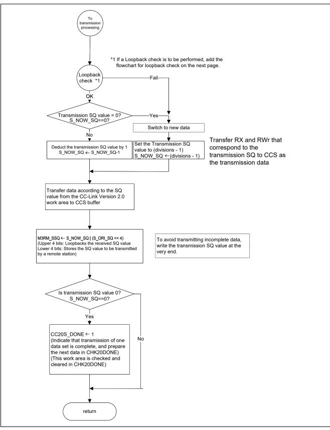
Figure 12.6 Transmission/Reception Processing Module ICCV20 (Continued 2)
