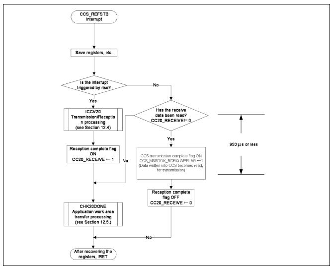
Figure 12.2 Transmission/Reception Processing Using Interrupt (CCS\_REFSTB Signal)
