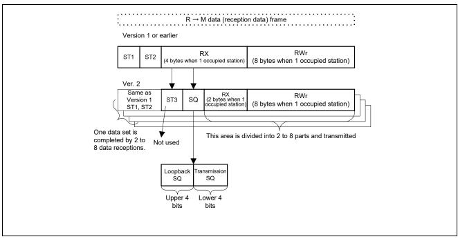
Figure 11.4 Details of SQ Value ( $R \rightarrow M$  Data)
