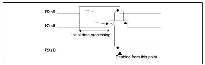
Figure 10.2 RXs9/RYs9 (Initial Data Processing Request / Processing Complete Flag)
