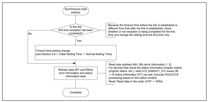
Figure 9.4 Synchronous Read Method
