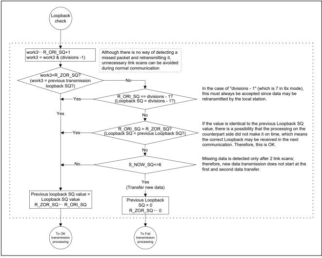
Figure 12.7 Transmission/Reception Processing Module ICCV20 (Continued 3)
