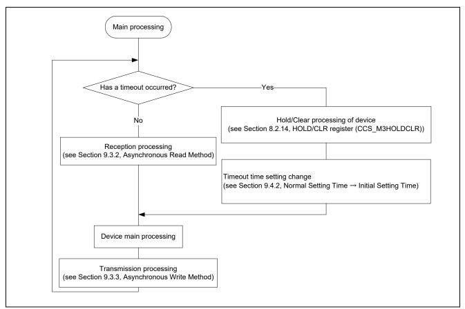
Figure 9.3 Asynchronous Read Method / Asynchronous Write Method
