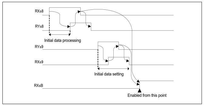
Figure 10.4 When Both RXs8/RYs8 and RXs9/RYs9 are Implemented
