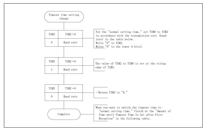
Figure 9.7 Initial Setting Time  $\rightarrow$  Normal Setting Time
