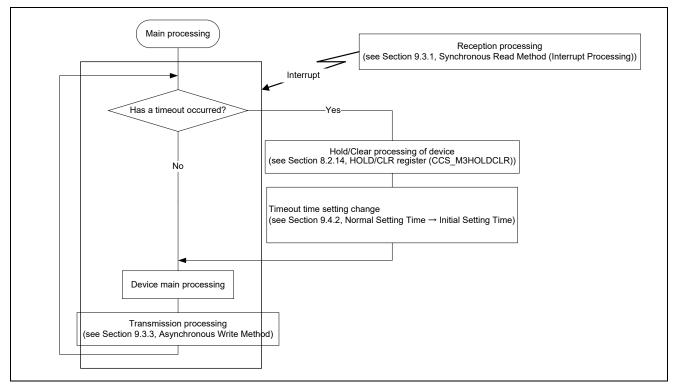
Figure 9.2 Synchronous Read Method / Asynchronous Write Method
