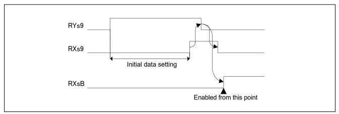
Figure 10.3 RXs9/RYs9 (Initial Data Setting Complete / Setting Request Flag)
