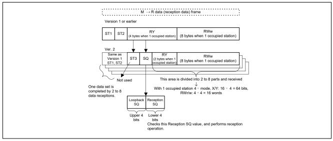
Figure 11.3 Details of SQ Value ( $M \rightarrow R$  Data)
