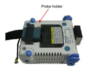
Figure 2-5. Connect the QB-RL78D1A2 to the probe
