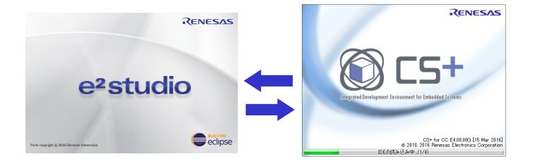
Existing projects can be converted between e<sup>2</sup> studio and CS+ through the project import and export functions although there are some restrictions due to the differences in project management policies between the tools.
