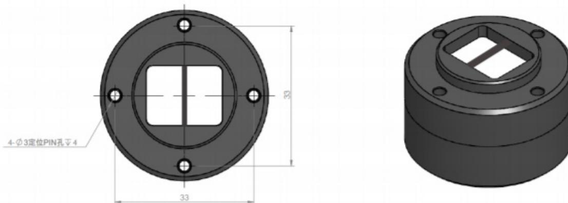
Figure 10. WhaleTeq Test Head with Optical Divider
