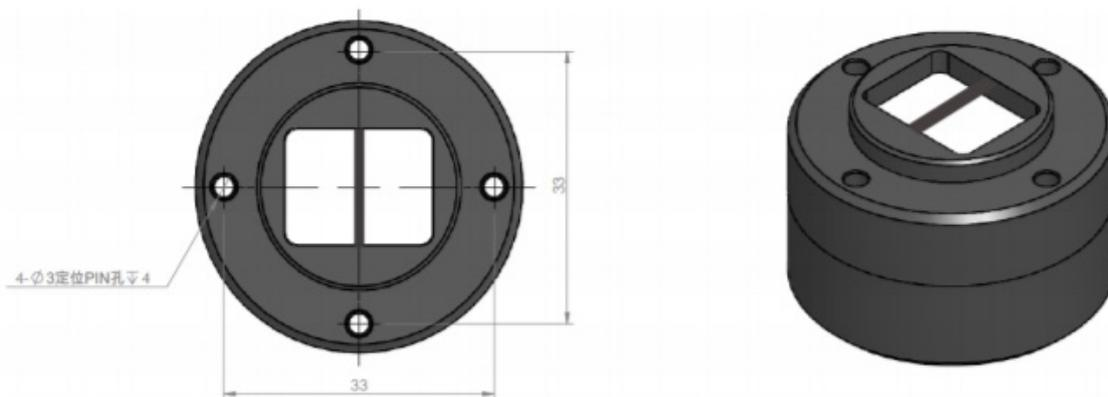
Figure 3. Mechanical Drawing of Fixture Base PPG-2R
