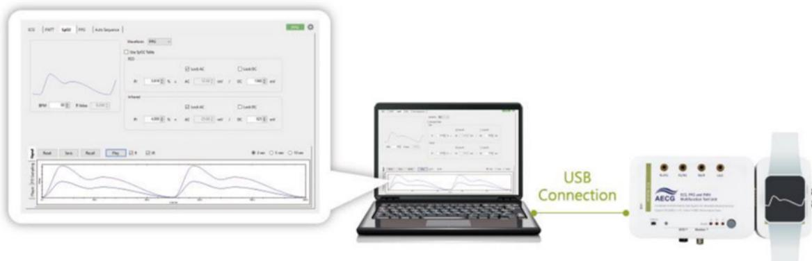
Figure 1. SP02 Test Setup with WhaleTeq AECG100
