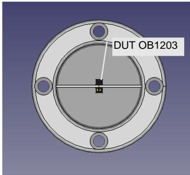
Figure 4. Top View of the OB1203 to WhaleTeq Test Adapter
