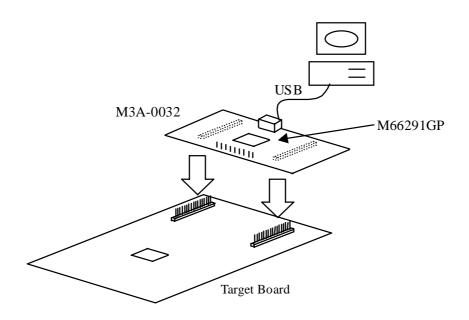
Figure 2 Target Board Connection Direction
