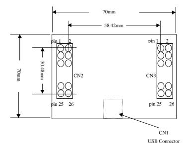
Figure 4 Pin Direction of Connector CN2 and CN3 (Bottom View)
