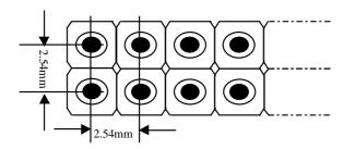
Figure 3 Pin Pitch of Connectors CN2 and CN3
