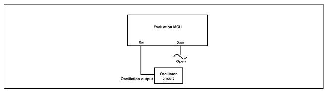
Figure 2.25 External oscillator circuit
