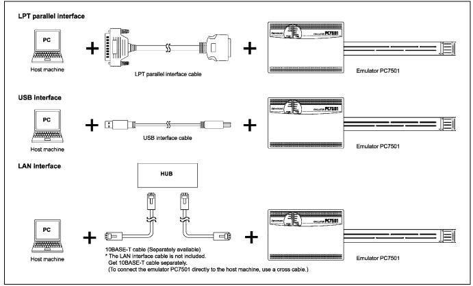
Figure 2.2 Outline for interface cable connections
