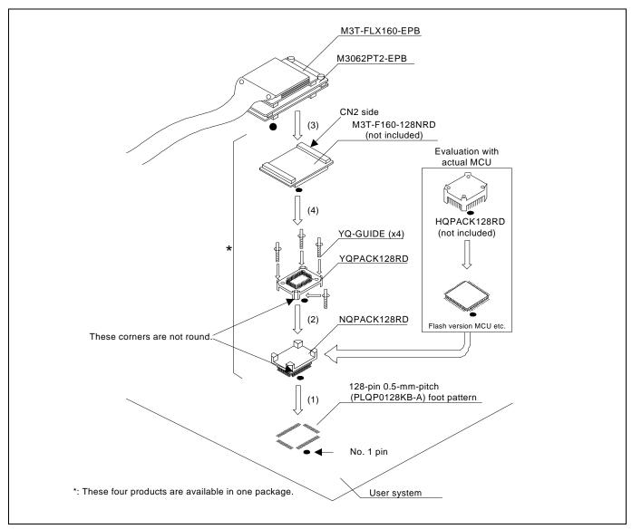
Figure 2.17 Connecting to a 128-pin 0.5-mm-pitch foot pattern
