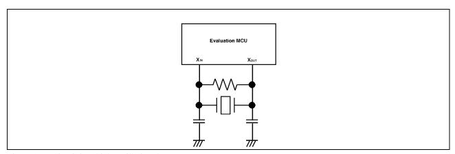
Figure 2.26 Circuit in which oscillation does not occur
