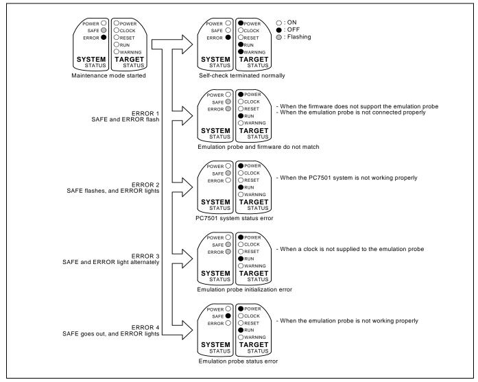
Figure 2.6 LED displays in the self-check
