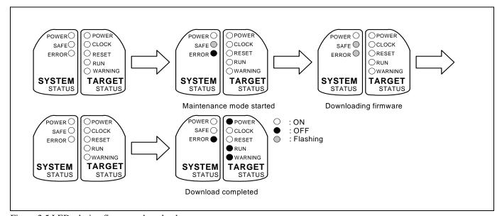
Figure 2.5 LEDs during firmware download
