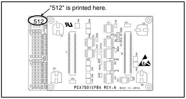
Figure 1.1 Printed area on the M3062PT2-EPB
