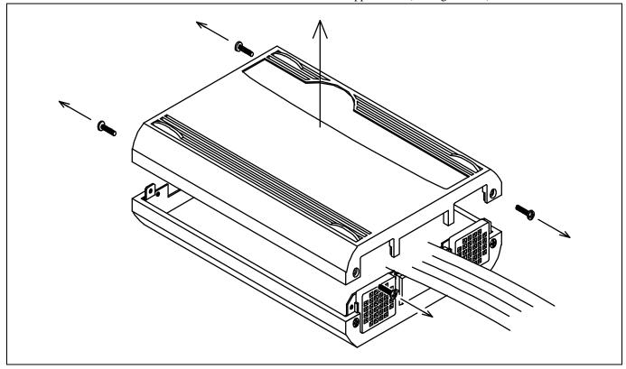
Figure 2.21 Removing the upper cover
