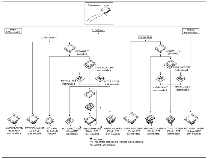
Figure 2.7 Connecting the user system according to user system
