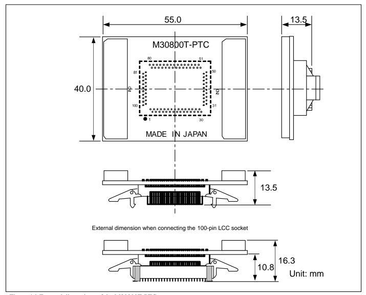
Figure 4.9 External dimensions of the M30800T-PTC
