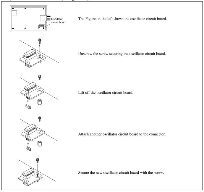
Figure 2.22 Replacing the oscillator circuit board
