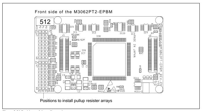
Figure 2.20 Positions of the pullup resistors
