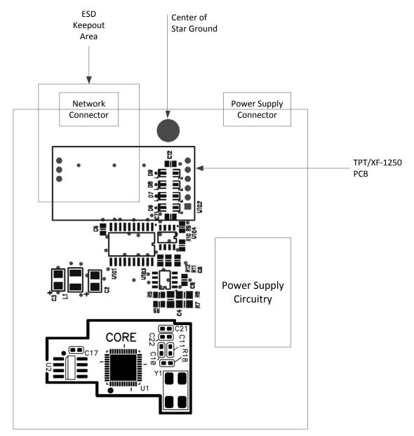
information about PCB layout and electromagnetic compatibility (EMC) design guidelines for a Series 5000 Chip, including the Router 5000.
