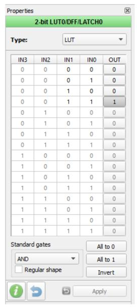
Figure 13: Look Up Table Properties Configured as an AND Gate
