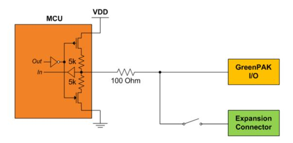
Figure 7: Schematic Connection of the Data Pin
