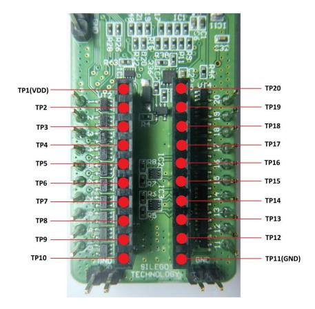
**Figure 2: DIP Adapter Connector Pinout**
