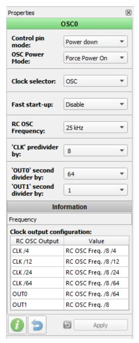
**Figure 16: Oscillator Properties**
