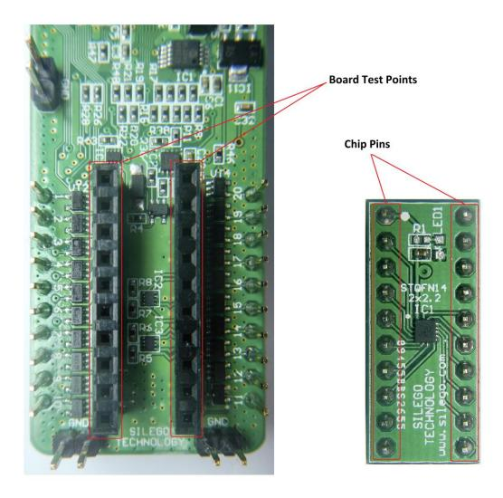
Figure 8: Pins and TPs Location
