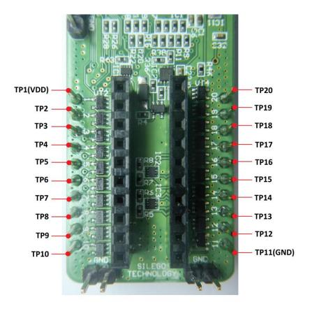
**Figure 4: Expansion Connector Pinout**
