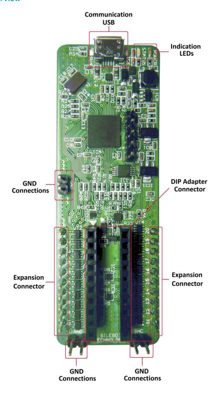
Figure 1: GreenPAK DIP Development Board, Top View
