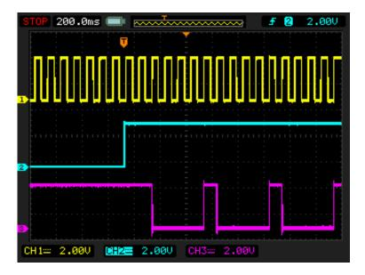
Figure 20: Waveform, Triggered on Button Pressed
