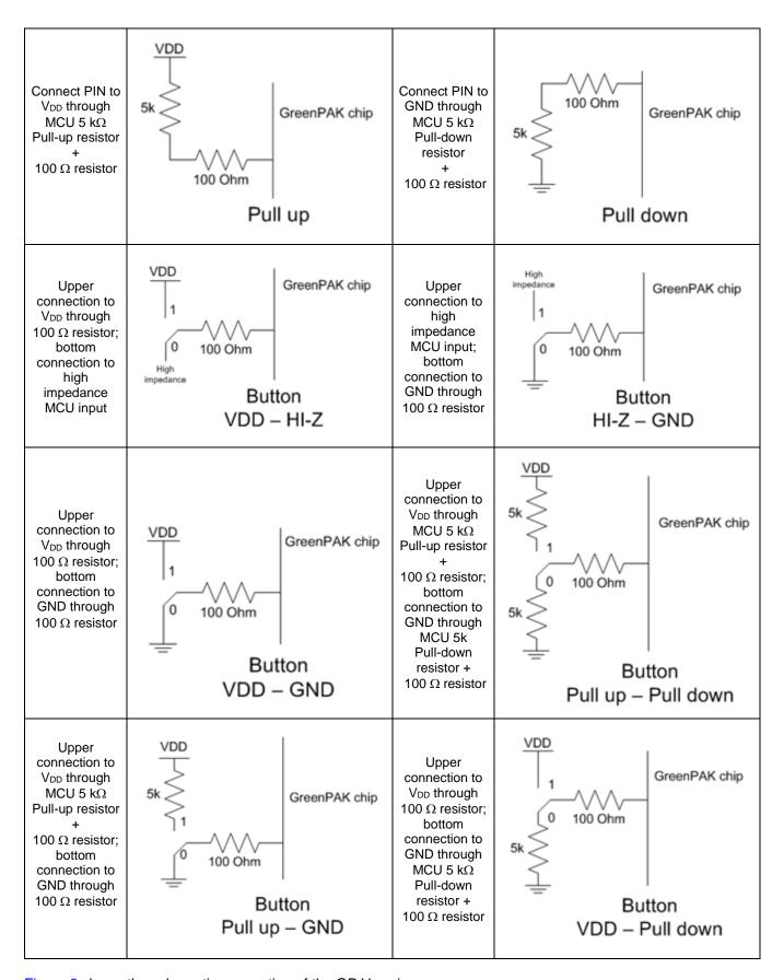
Figure 6 shows the schematic connection of the GP V<sub>DD</sub> pins.
