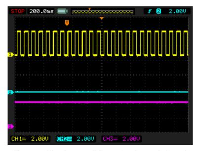
Figure 21: Waveform, no Triggered on Button Released
