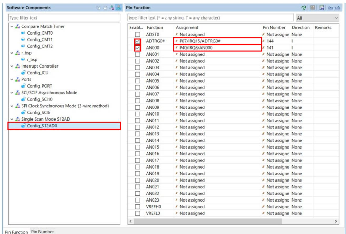
**Figure 4-53 Configure pin assignment - Config\_S12AD0**
