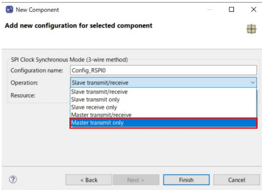
**Figure 4-39 Select Operation – Master transmit only**
