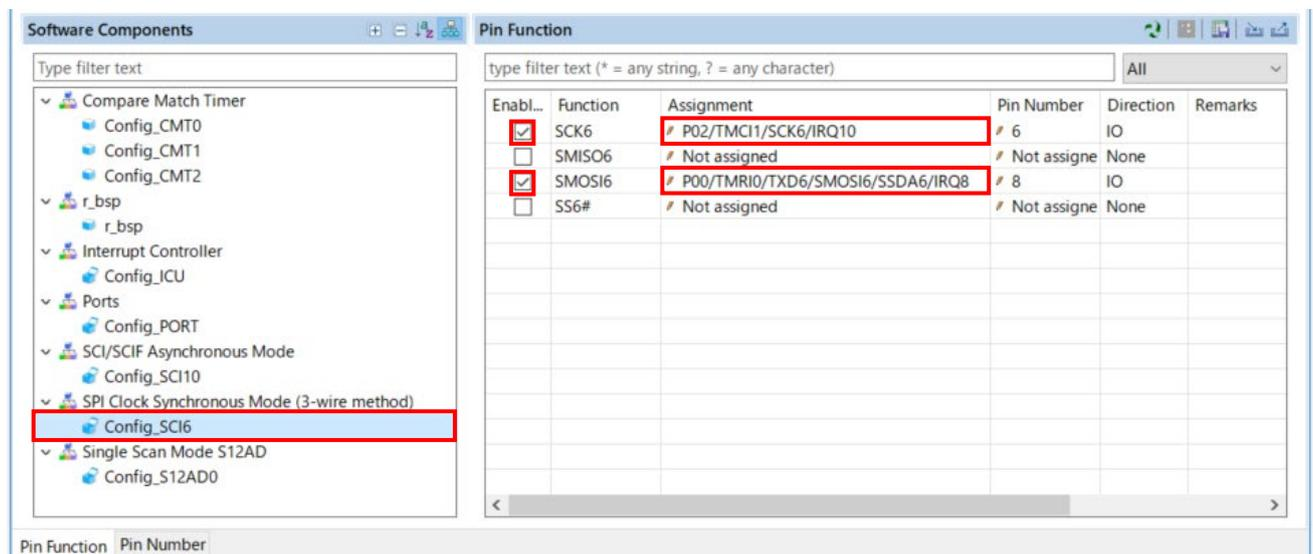
**Figure 4-52 Configure pin assignment - Config\_SCI6**
