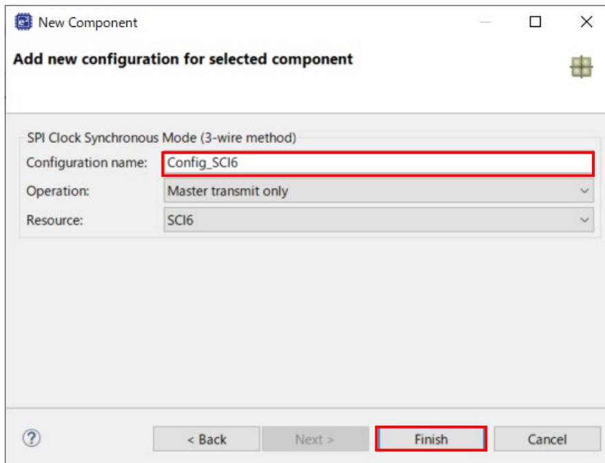
**Figure 4-41 Ensure Configuration name - Config\_SCI6**
