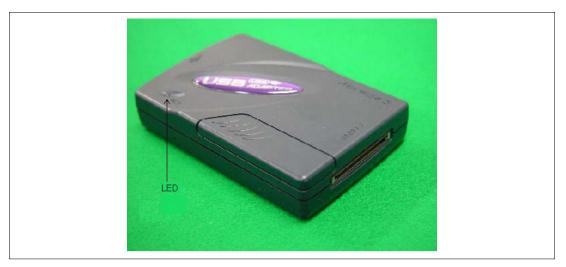
Figure 5.1 LED for Displaying the Communication State
