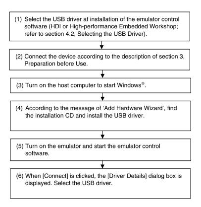
Figure 4.1 Setup Procedures
