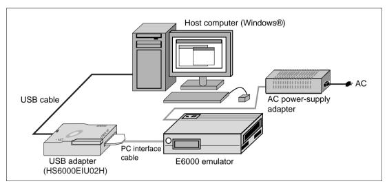
Figure 1.1 System Configuration of E6000 Emulator Connection
