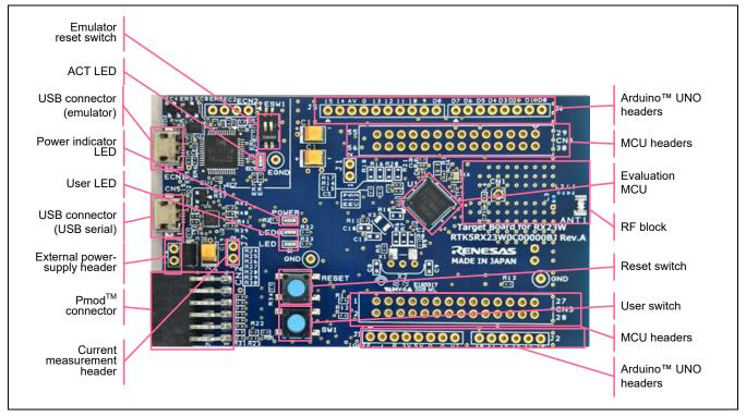
Figure 2-1 Board Layout (Top Side)
