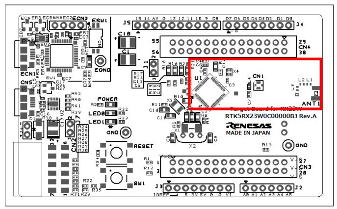
Figure 5-1 BLE Circuit
