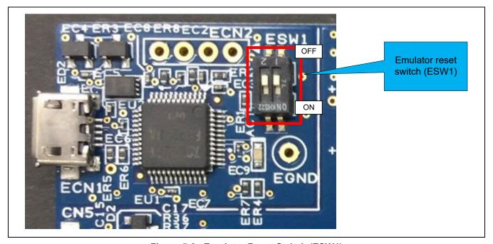
Figure 5-2 Emulator Reset Switch (ESW1)
