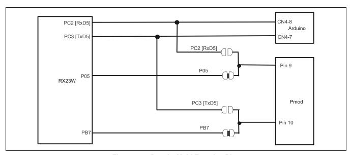
Figure 5-7 Pmod™ Multi-Function Pins
