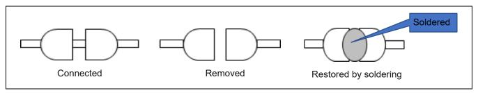
Figure 5-9 Examples of States of Patterns for Cutting
