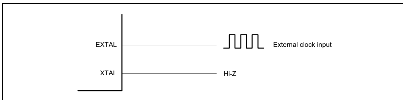
Figure 9.5 Equivalent circuit for external clock
