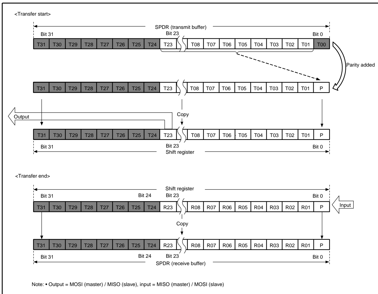
Figure 35.20 MSB-First Transfer (24-Bit Data, Parity Enabled)
