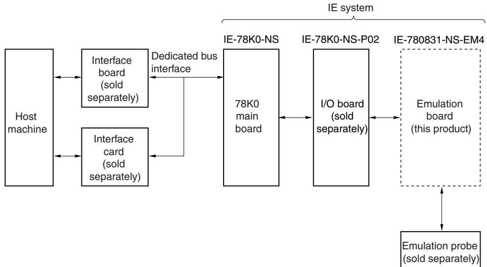
**Figure 1-3. Basic Hardware Configuration (Using IE-78K0-NS-A)**
