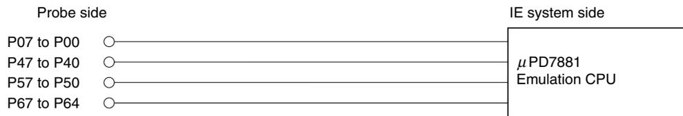
Figure 4-3. Equivalent Circuit of Emulation Circuit 3
