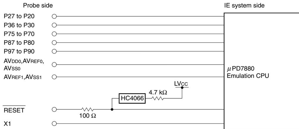
Figure 4-2. Equivalent Circuit of Emulation Circuit 2
