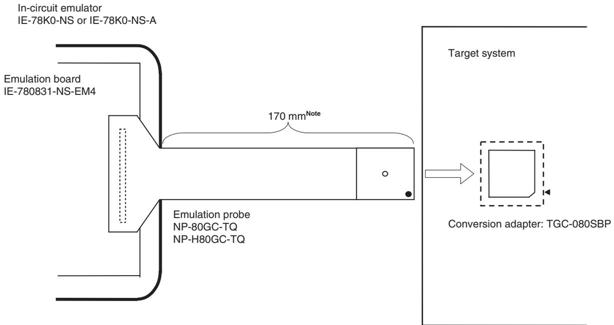
**Note** Distance when NP-80GC-TQ is used. When NP-H80GC-TQ is used, the distance is 370 mm.
