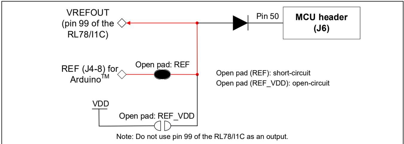
Figure 5-26 Circuit Schematic when REF for Arduino™ is Selected
