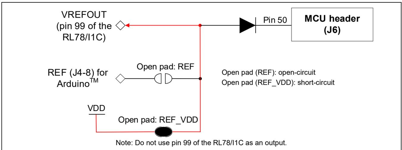
Figure 5-27 Circuit Schematic when VDD is Selected
