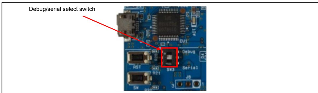
Figure 5-14 Position of the Debug/Serial Select Switch (Top Side)
