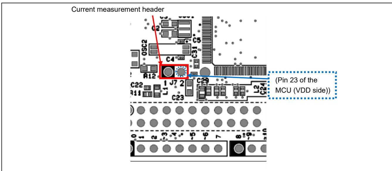
Figure 5-21 Position of the Current Measurement Header (Top Side)
