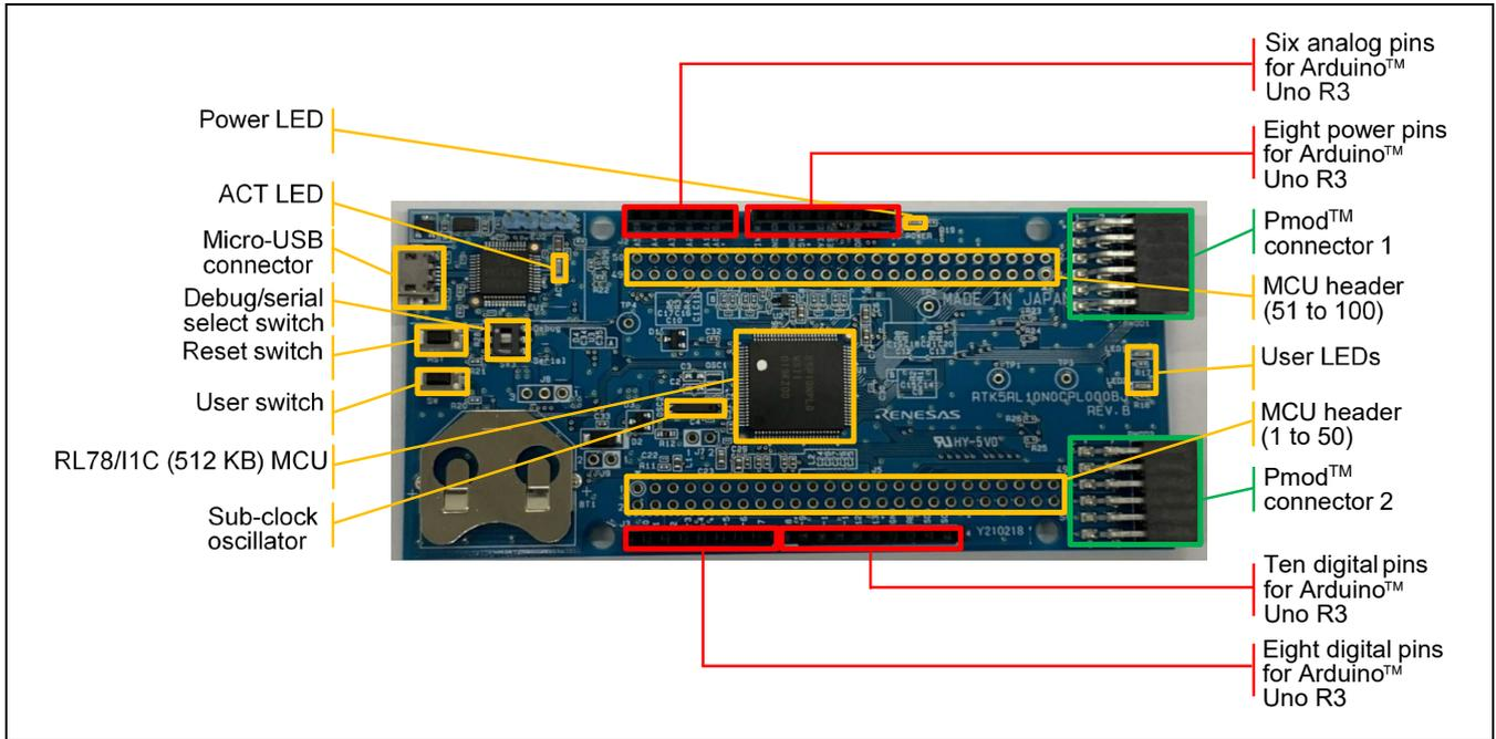
Figure 2-1 Board Layout (Top Side)
