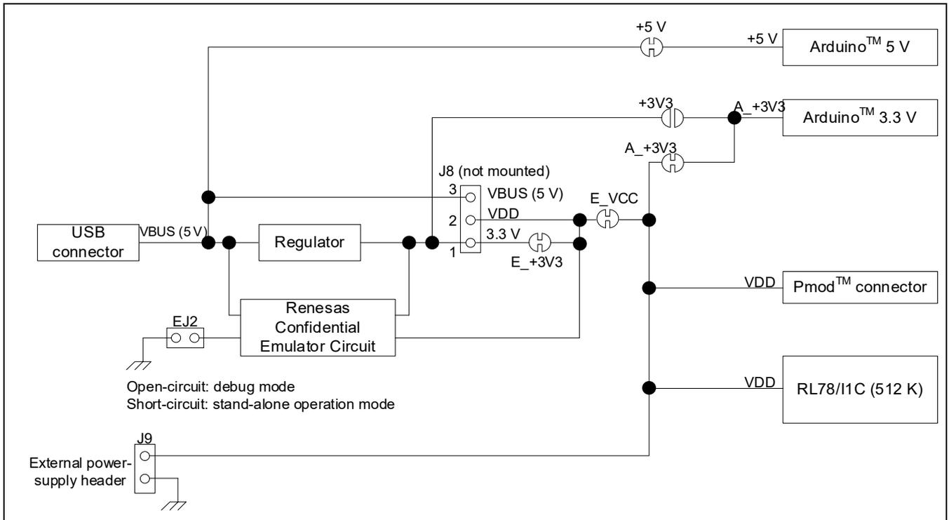
Figure 6-1 Block Diagram of the Power-Supply Circuit
