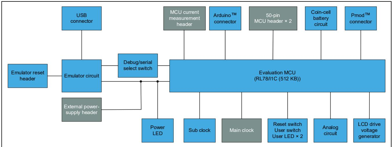
Figure 1-1 Block Diagram
