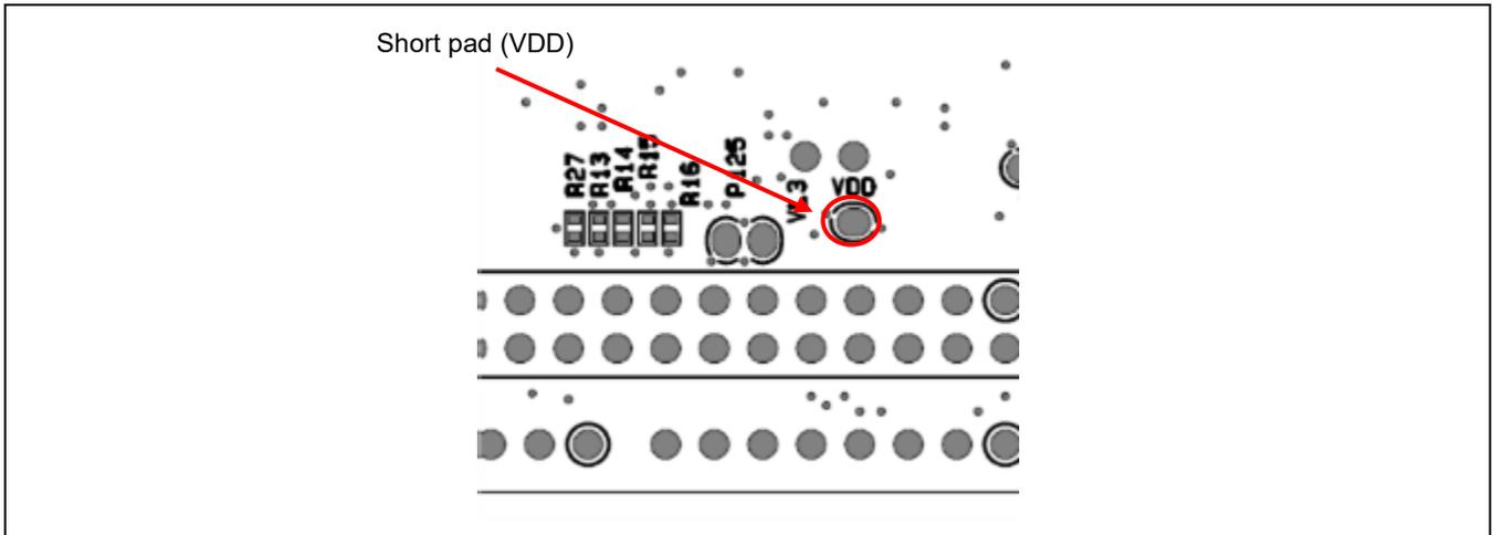
**Figure 5-22 Position of the Short Pad (VDD) (Soldered Side)**
