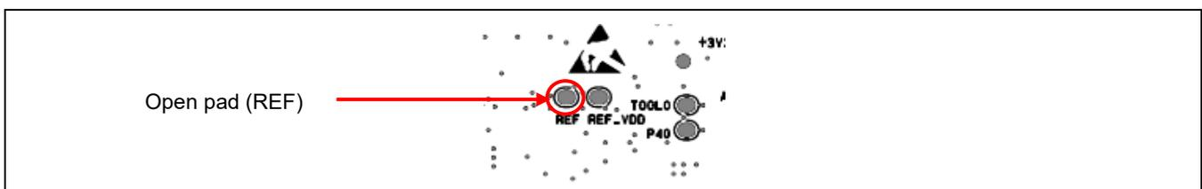
**Figure 5-7 Position of the Open Pad (REF) (Soldered Side)**
