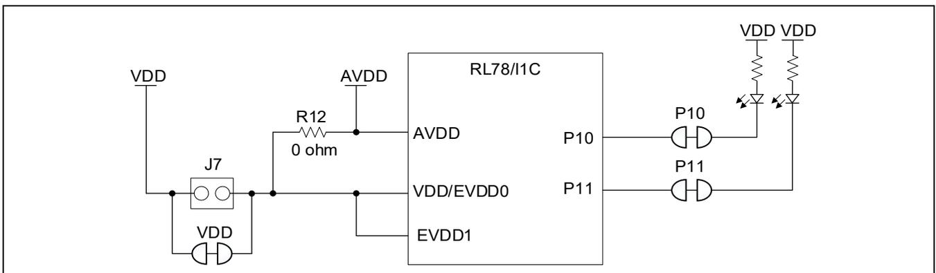
**Figure 5-23 Block Diagram of the Headers Related to MCU Current Measurement**
