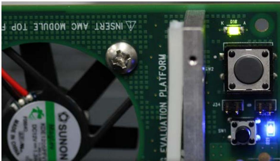
LED D1 Indicates the link between the host PC and Tsi721 is active.
