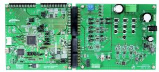
**RA6T2 CPU Board and Inverter Board**
