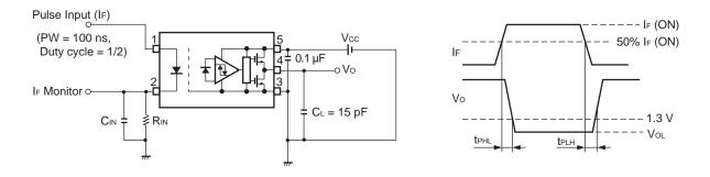
Remark C<sub>L</sub> includes probe and stray wiring capacitance.
