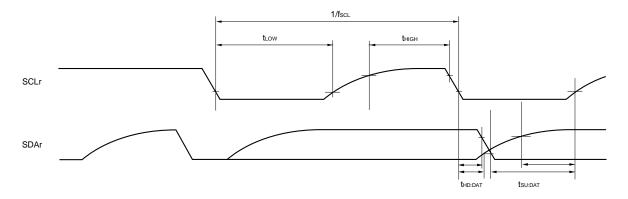
Caution Select the TTL input buffer and the N-ch open drain output (EV<sub>DD</sub> tolerance) mode for the SDAr pin and the N-ch open drain output (EV<sub>DD</sub> tolerance) mode for the SCLr pin by using port input mode register g (PIMg) and port output mode register g (POMg). For V<sub>IH</sub> and V<sub>IL</sub>, see the DC characteristics with TTL input buffer selected.
