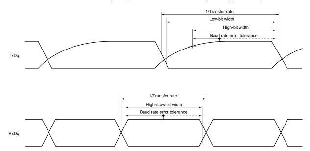
Caution Select the TTL input buffer for the RxDq pin and the N-ch open drain output (EVDD tolerance) mode for the TxDq pin by using port input mode register g (PIMg) and port output mode register g (POMg). For VIH and VIL, see the DC characteristics with TTL input buffer selected.
