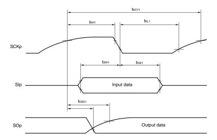
Caution Select the TTL input buffer for the SIp pin and the N-ch open drain output (EVDD tolerance) mode for the SOp pin and SCKp pin by using port input mode register g (PIMg) and port output mode register g (POMg). For VIH and VIL, see the DC characteristics with TTL input buffer selected.
