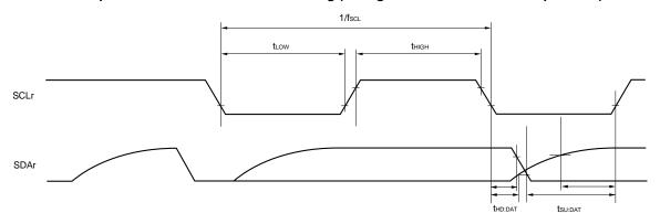
Caution Select the normal input buffer and the N-ch open drain output (EVDD tolerance) mode for the SDAr pin and the normal output mode for the SCLr pin by using port input mode register g (PIMg) and port output mode register g (POMg).
