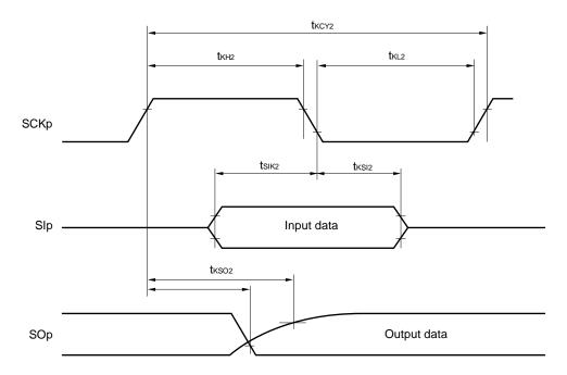
Caution Select the TTL input buffer for the SIp pin and SCKp pin and the N-ch open drain output (EVDD tolerance) mode for the SOp pin by using port input mode register g (PIMg) and port output mode register g (POMg). For V<sub>IH</sub> and V<sub>IL</sub>, see the DC characteristics with TTL input buffer selected.
