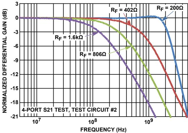
FIGURE 16. SMALL SIGNAL RESPONSE vs GAIN
