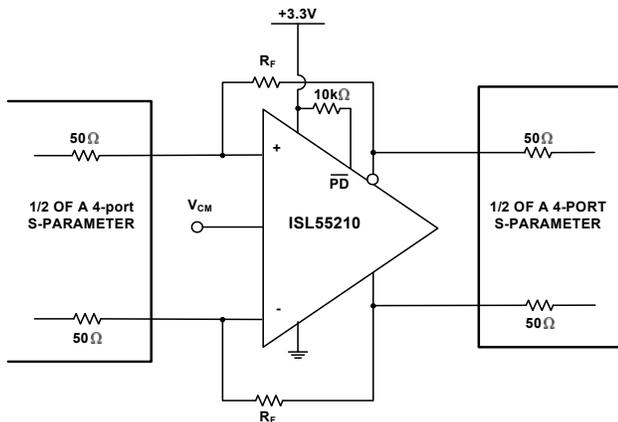
FIGURE 29. TEST CIRCUIT #2 4-PORT S-PARAMETER MEASUREMENTS
