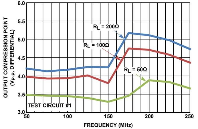
FIGURE 5. OUTPUT  $V_{p-p}$  FOR -1dB GAIN COMPRESSION
