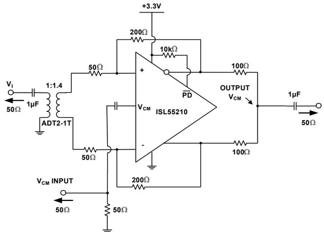
FIGURE 30. TEST CIRCUIT #3 COMMON MODE AC OUTPUT MEASUREMENTS
