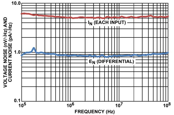
FIGURE 15. INPUT VOLTAGE AND CURRENT SPOT NOISE
