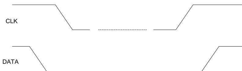
**Figure 18: Timing of START and STOP Condition**
