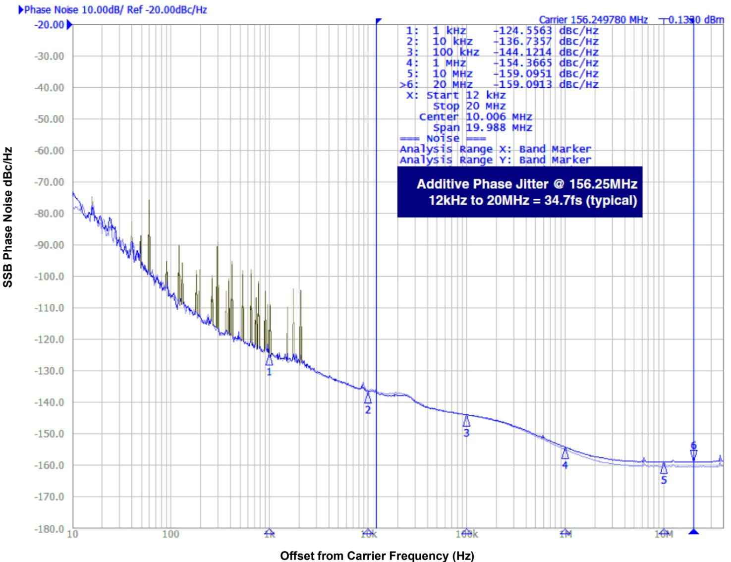
As with most timing specifications, phase noise measurements have issues relating to the limitations of the measurement equipment. The noise floor of the equipment can be higher or lower than the noise floor of the device. Additive phase noise is dependent on both the noise floor of the input source and measurement equipment.
