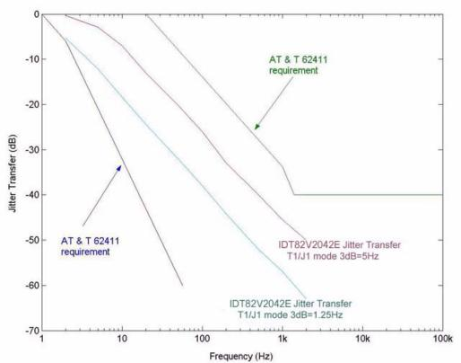
Figure-28 T1/J1 Jitter Transfer Performance
