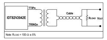
Figure-6 T1 Pulse Template Test Circuit
