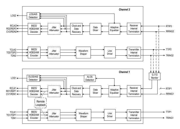
Figure-11 G.772 Monitoring Diagram
