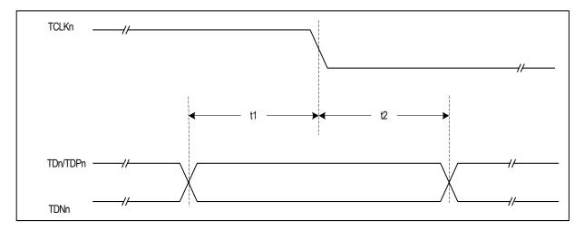
Figure-23 Transmit System Interface Timing
