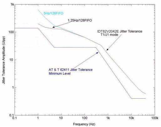
Figure-26 T1/J1 Jitter Tolerance Performance
