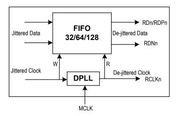
Figure-12 Jitter Attenuator
