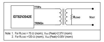
Figure-4 E1 Pulse Template Test Circuit
