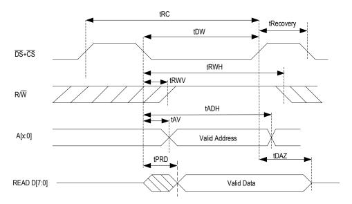
Figure-33 Non-Multiplexed Motorola Read Timing
