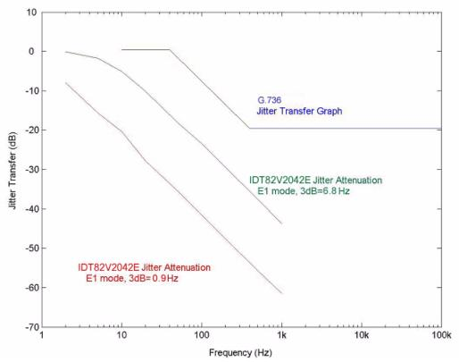
Figure-27 E1 Jitter Transfer Performance
