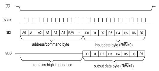
Figure-20 Serial Microcontroller Interface Function Timing
