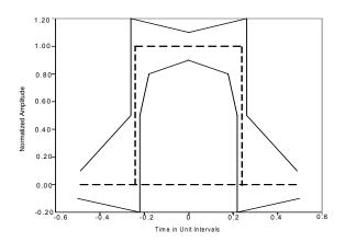
Figure-3 E1 Waveform Template Diagram
