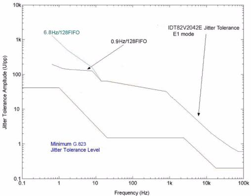
Figure-25 E1 Jitter Tolerance Performance
