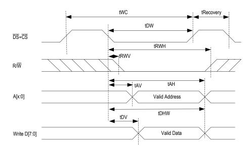
Figure-34 Non-Multiplexed Motorola Write Timing
