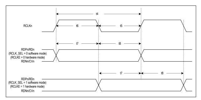
Figure-24 Receive System Interface Timing
