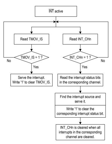
Figure-29 Interrupt Service Process
