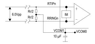
Note: 1. Two Rr/2 resistors should be connected to VCOM[1:0] that are coupled to ground via a 10  $\mu$ F capacitor, which provide 60  $\Omega$ common mode input resistance.
