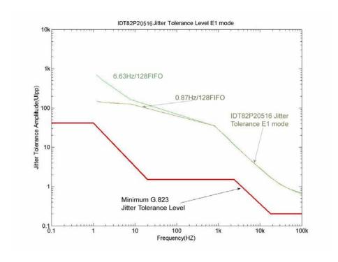
Figure-39 E1 Jitter Tolerance Performance
