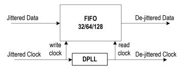
Figure-14 Jitter Attenuator
