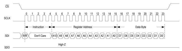
Figure-42 Write Operation in Serial Microprocessor Interface
