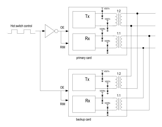
Rx: Fully Internal Impedance Matching mode. In this mode, there is no external resistor required. The R\_TERM[2:0] bits (b2~0, RCF0,...) setting is as follows: '010' for E1 120  $\Omega$  twisted pair cable and '011' for E1 75  $\Omega$  coaxial cable.
