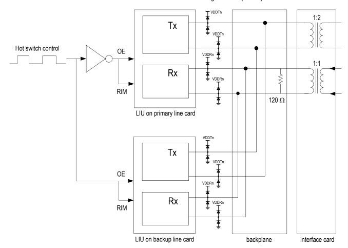
**Rx:** Partially Internal Impedance Matching mode. A fixed external 120  $\Omega$  resistor is placed on the backplane and provides a common termination for E1 applications. The R\_TERM[2:0] bits (b2~0, RCF0,...) setting is as follows: '010' for E1 120  $\Omega$  twisted pair cable and '011' for E1 75  $\Omega$  coaxial cable.
