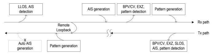
Figure-24 Priority Of Diagnostic Facilities During Manual Remote Loopback
