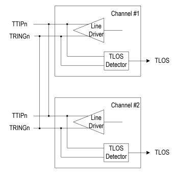
Figure-16 TLOS Detection Between Two Channels
