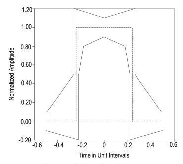
Figure-9 E1 Waveform Template
