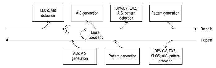
Figure-25 Priority Of Diagnostic Facilities During Digital Loopback
