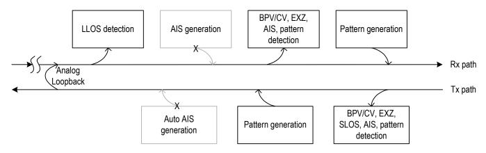
Figure-23 Priority Of Diagnostic Facilities During Analog Loopback
