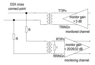
Figure-8 Transmit Path Monitoring
