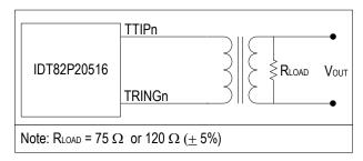
Figure-10 E1 Waveform Template Measurement Circuit
