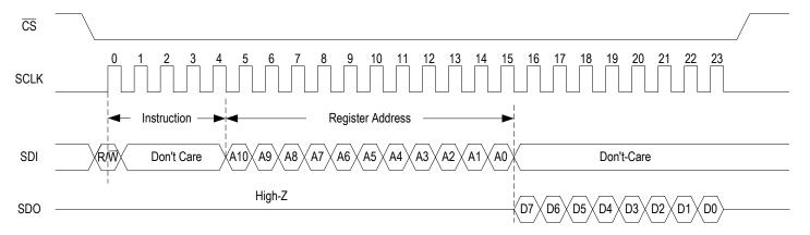
Figure-41 Read Operation in Serial Microprocessor Interface
