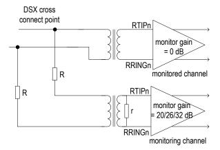
Figure-7 Receive Path Monitoring
