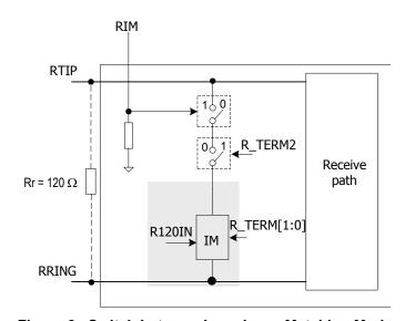
Figure-3 Switch between Impedance Matching Modes
