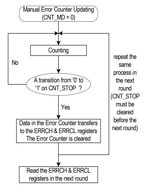
Figure-22 Manual Error Counter Updating
