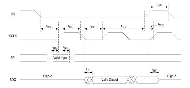
Figure-43 Timing Diagram
