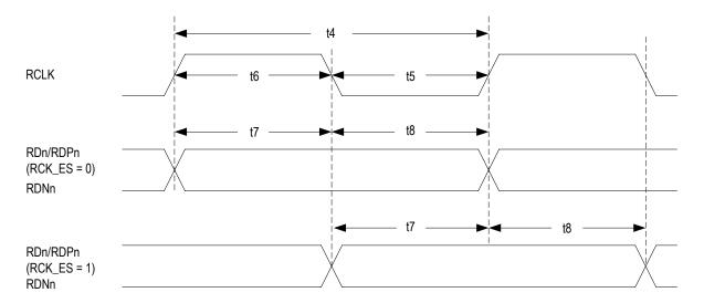
Figure-37 Receive Clock Timing Diagram
