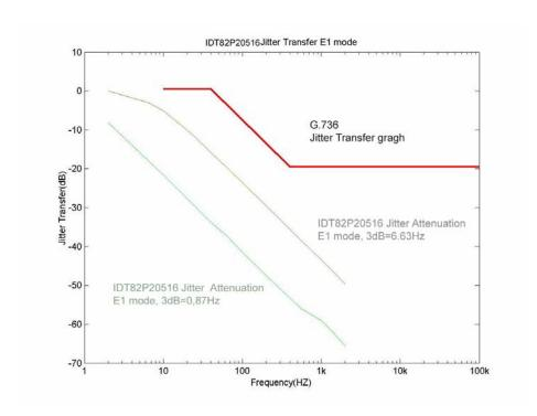
Figure-40 E1 Jitter Transfer Performance
