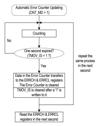
Figure-21 Automatic Error Counter Updating
