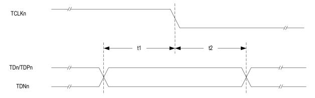
Figure-36 Transmit Clock Timing Diagram
