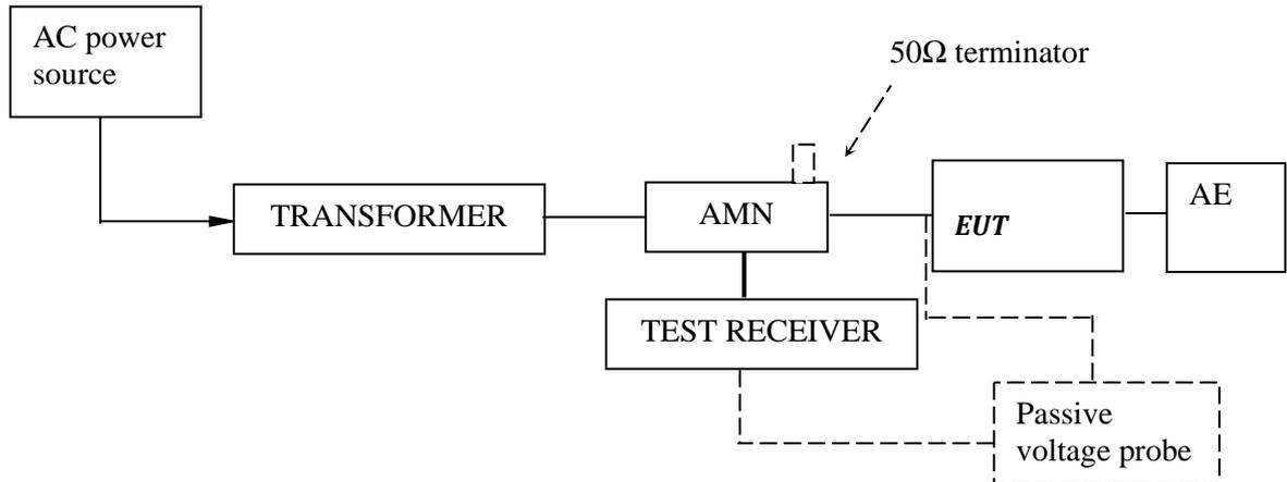
Test Setup and Procedure:
