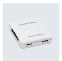
On-chip debugging emulator with programmer function
